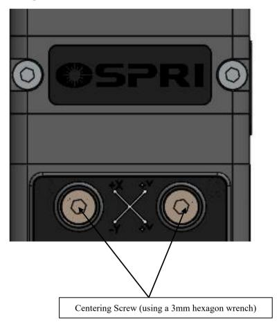
Relationship between Beam Position and Adjustment Knobs:
