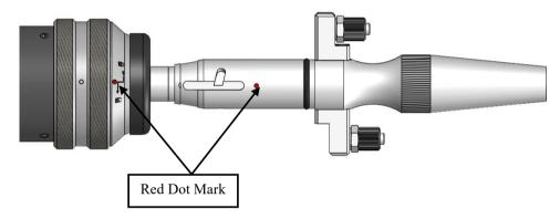
⑤ Twist the QBH connector to the locked position: Rotate it clockwise to the extreme position (you can feel a "click" sound), then lift up the rotating nut and rotate it clockwise again until the fiber optic head is securely pressed down. (Note: Only rotate it to the proper position and avoid excessive force, as it may damage the internal structure.)
